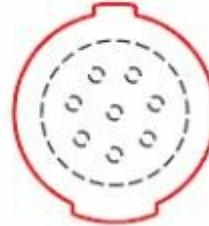
**Insert:** The male and female insert can be assembled in all three housings.
