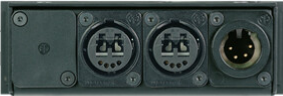
Rear view: e.g. 2R (opticalCON DUO)
