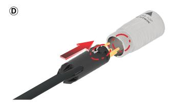
(D) Slide insert and chuck together into the housing.
