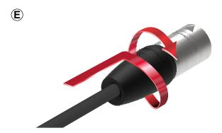
(E) Finish the installation by turning the bushing onto the connector.
